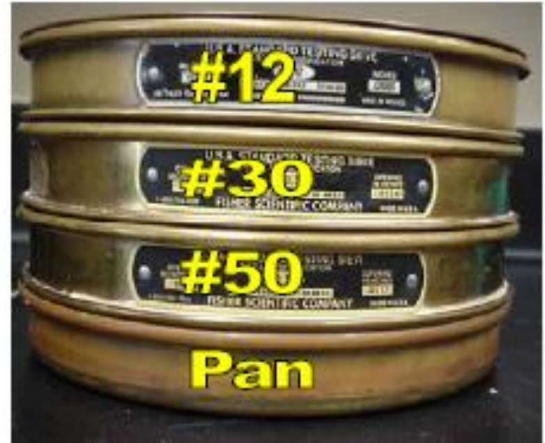
Step 3: Stack sieves in proper order.
