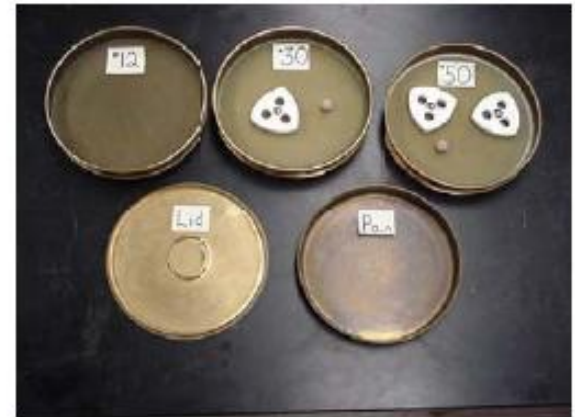
Step 1: Prepare sieves with appropriate number of balls and carnucle brushes.
