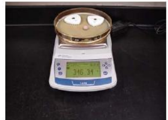
Step 2: Weigh each empty sieve along with its ball and carnucle(s).
