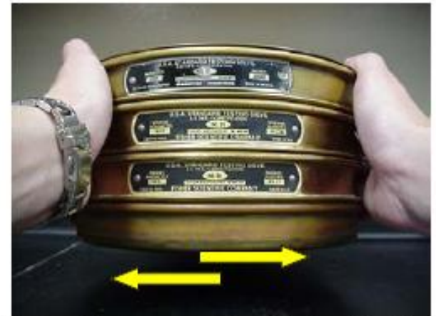
Step 5: Shake sample side to side for 90 seconds.
